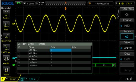
Figure 7-2 Parallel Decoding Event Table
