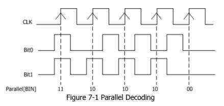
Press **MATH**  $\rightarrow$  **Decode1**  $\rightarrow$  **Decoder** to select "Parallel" and open the parallel decoding function menu.
