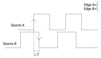
Figure 5-10 Delay Trigger
