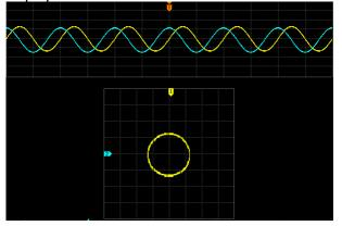
Observe the measurement result shown in the figure above. According to the measurement schematic diagram of the phase deviation (as shown in Figure 3-2), A/B (C/D) = 1. Thus, the phase deviation angle θ=±arcsin1=90°.
