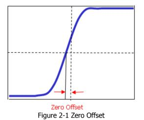
Press **CH1**  $\rightarrow$  **Delay-Cal** and use  $\checkmark$  to set the desired delay time. The range available is from -100 ns to 100 ns. Pressing down the multifunction knob  $\checkmark$  will reset the delay time to 0.00 s.
