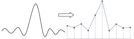
2. **Waveform Confusion:** when the sample rate is lower than twice the actual signal frequency (Nyquist Frequency), the frequency of the waveform rebuilt from the sample data is lower than the actual signal frequency.
