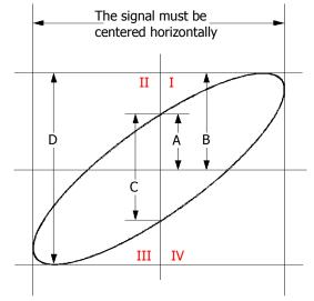
Figure 3-2 Measurement Schematic Diagram of Phase Deviation
