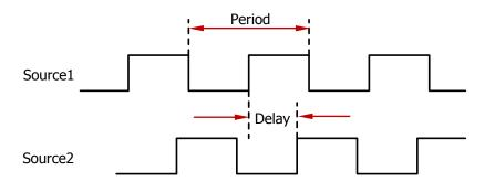
Figure 6-4 Delay and Phase
