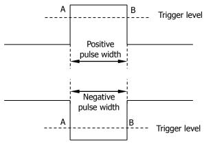
Figure 5-3 Positive Pulse Width/Negative Pulse Width
