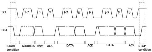
Figure 5-14 Schematic Diagram of I2C Protocol
