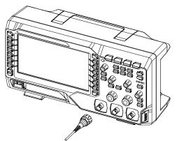
Figure 1-5 To Connect the Passive Probe
