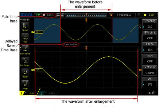
Figure 3-1 Delayed Sweep Mode
