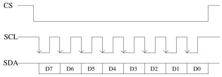
Figure 5-15 Sequential Chart of SPI Bus
