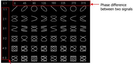
Frequency ratio between two signals
