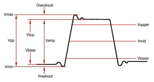
Figure 6-5 Voltage Parameters
