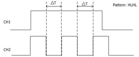
Figure 5-7 Duration Trigger
