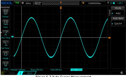
The following figure shows the auto measurement example of sine signal frequency in CH2.
