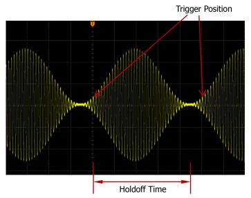
Figure 5-2 Schematic Diagram of Trigger Holdoff
