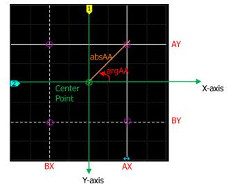
Figure 6-8 XY Cursor Measurement Definition
