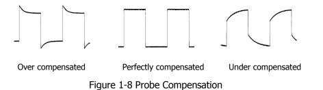
3. Use a nonmetallic driver to adjust the low-frequency compensation adjustment hole on the probe until the displayed waveform is displayed as "Perfectly compensated" in the figure above.
