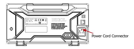
Figure 1-4 To Connect to Power Supply
