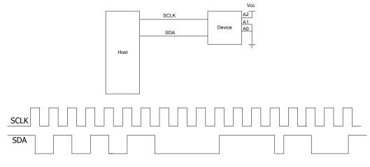
Figure 7-5 I2C Serial Bus
