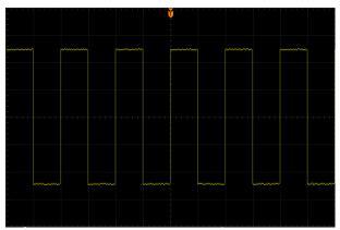
Figure 4-2 The Waveform after 256 Averages
