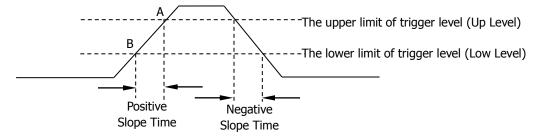
Figure 5-4 Positive Slope Time/Negative Slope Time
