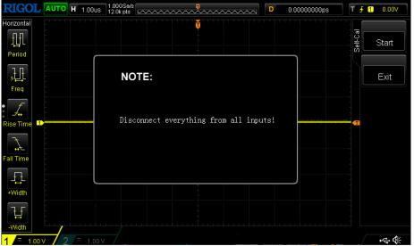
Figure 13-2 Self-calibration Interface
