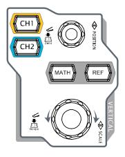
**CH1**, **CH2**: analog channel setting keys. The 2 channels are marked by different colors which are also used to mark both the corresponding waveforms on the screen and the channel input connectors. Press any key to open the corresponding channel menu and press again to turn off the channel.
