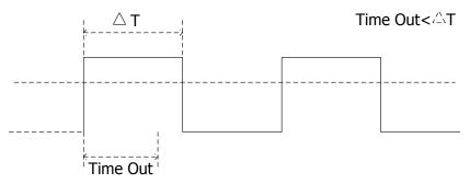
Figure 5-8 TimeOut Trigger
