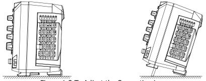
Figure 1-3 To Adjust the Supporting Legs
