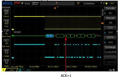
Figure 7-7 I2C Error Expressions during Decoding
