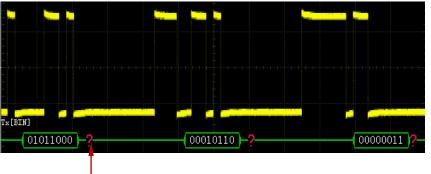
The stop bit is less than 1
