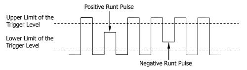
Figure 5-9 Runt Trigger
