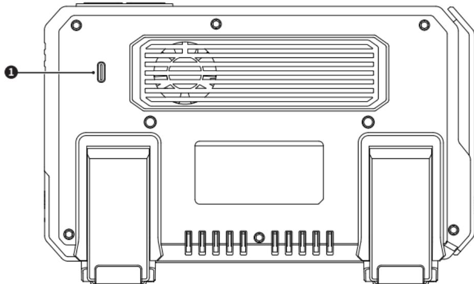
① **Power port:** Power interface, supports Type-C input with fast charging protocol, rated at 12V, **1A**.
